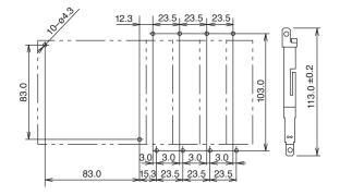
Mounting hole layout from left, FC4A-HPH1, FC4A-D20K3, FC4A-N16B3, FC4A-N32B3, and FC4A-M24BR2 modules
